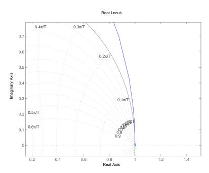
The locus (blue line) starts from the double pole at z=1 and goes outside the unit circle—this system is unstable.
