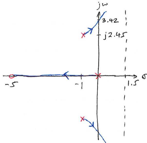
Figure 2: Root locus sketch for Problem 8, using asymptotes,  $j\omega$  axis crossing, and departure angles.
