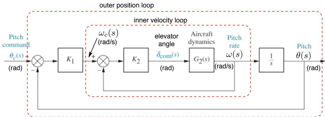
Figure 5: F4E Pitch Stabilization Loop.
