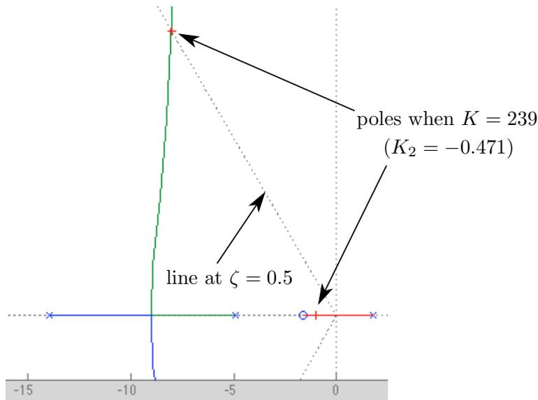
Figure 7: Root locus of inner loop for part (d).
