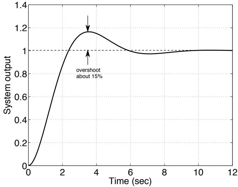
Figure 3: Unit step response for Problem 30 with  $K$  set for  $\zeta = 0.5$ .
