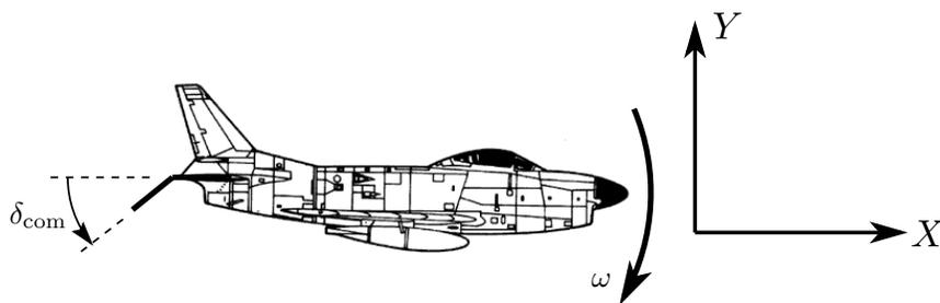
The aircraft elevator is shown with a positive displacement  $\delta_{com}$  (positive around  $Z$  axis by RH rule). By intuitive reasoning you can see that this elevator displacement will cause the aircraft to pitch **down**, as shown by the angular direction  $\omega$ .
