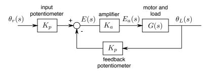
Let the transfer function of the "motor and load" be the G(s) of the Chapter 4 HW problem, with load position  $\theta_L$ in rad, and motor voltage  $e_a$  in V. Both the "input potentiometer" and "feedback potentiometer" are identical, and have transfer function (gain) of  $K_p$  V/rad in accordance with Chapter 1 Problem 1.
