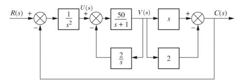
Starting from the "inside out"...first reduce the inner forward path V(s)/U(s), then the inner parallel blocks C(s)/V(s), then the outer feedback loop.
