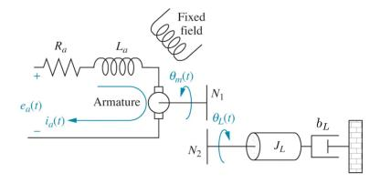
The specifications for the Pittman 7214 DC motor (taken from the manufacturer's data sheet) are:
