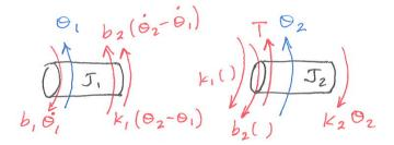
As I said in the "hints", the two moments on  $J_2$  labeled  $k_1()$  and  $b_2()$  are just  $k_1(\theta_2 - \theta_1)$  and  $b_2(\dot{\theta}_2 - \dot{\theta}_1)$ . To find the equations of motion (EOM), just apply  $\Sigma T = J\ddot{\theta}$  for each rotary inertia. The EOMs for both inertias are:
