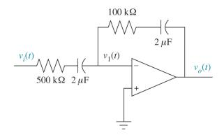
As I stated in class, an "inverting amplifier" circuit of this type with input impedance  $Z_i(s)$  and feedback impedance  $Z_f(s)$  will have TF
