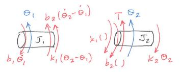
The two moments on  $J_2$  labeled  $k_1()$  and  $b_2()$  are just  $k_1(\theta_2 - \theta_1)$  and  $b_2(\dot{\theta}_2 - \dot{\theta}_1)...$  I didn't feel like writing them twice. The equation of motion I obtained for the second inertia was:
