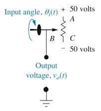
If it takes 10 turns to move the wiper arm from A to C, draw a block diagram of the potentiometer showing the input variable, the output variable, and (inside the block) the gain.
