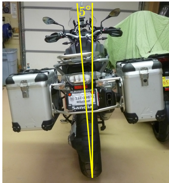
Figure 5: Bike lean of 5° with modified sidestand—perfect!
