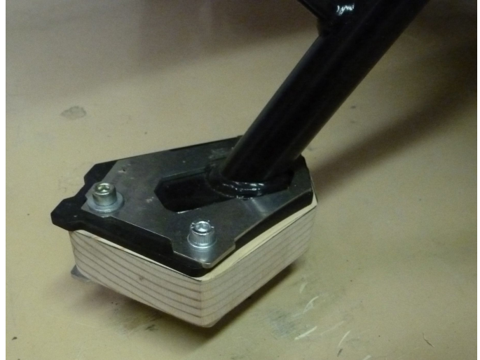
Figure 4: Unpainted 1-inch shim in place on side-stand.
