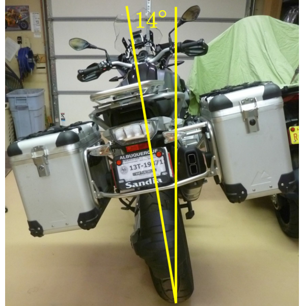
Figure 1: Bike lean of 14^\circ with original sidestand. This was a little too much for me.
