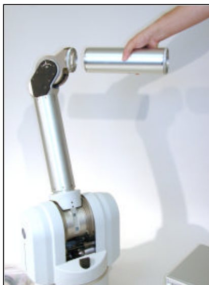
Figure 10 - Separating the Outer Link
